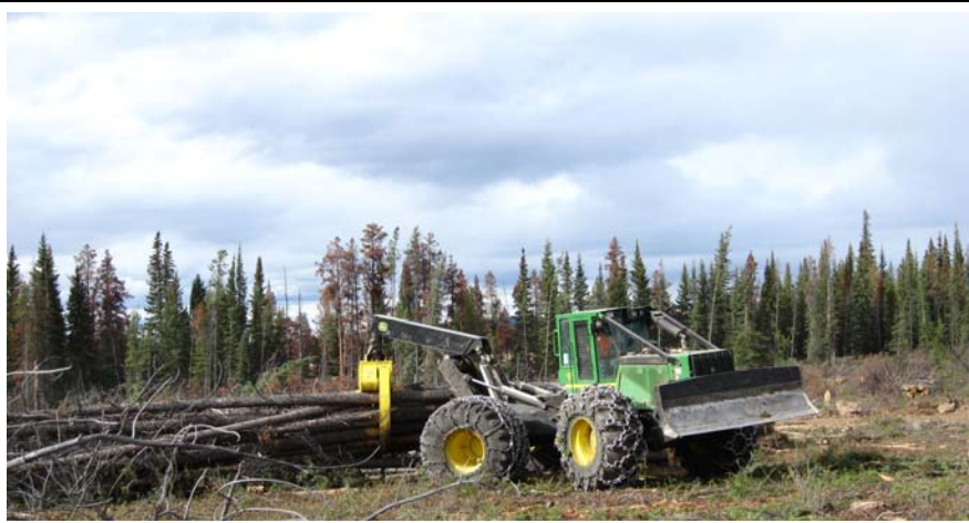
Photo #2: Grapple skidder skids a turn of pine to roadside where it will be further processed into predetermined cut to length (CTL) sawlogs and hauled to Williams Lake.
