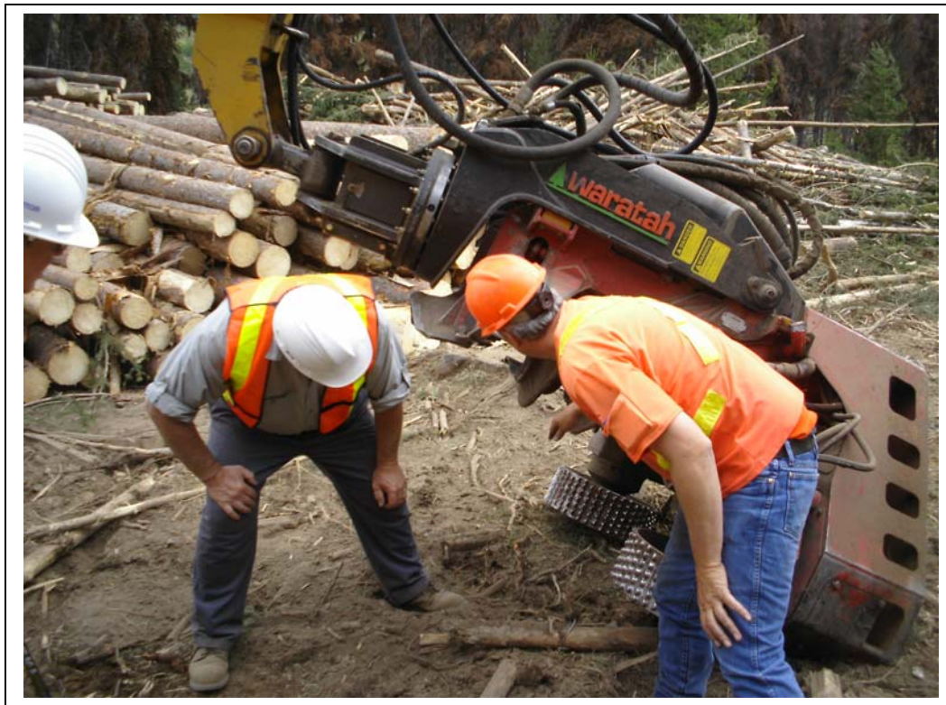
Photo #4: Public Advisory Member (white hat) gets a lesson in processor maintenance from the machine operator. During the inspection process particular attention is paid to cylinders and hoses where seals could leak hydraulic fluid.
