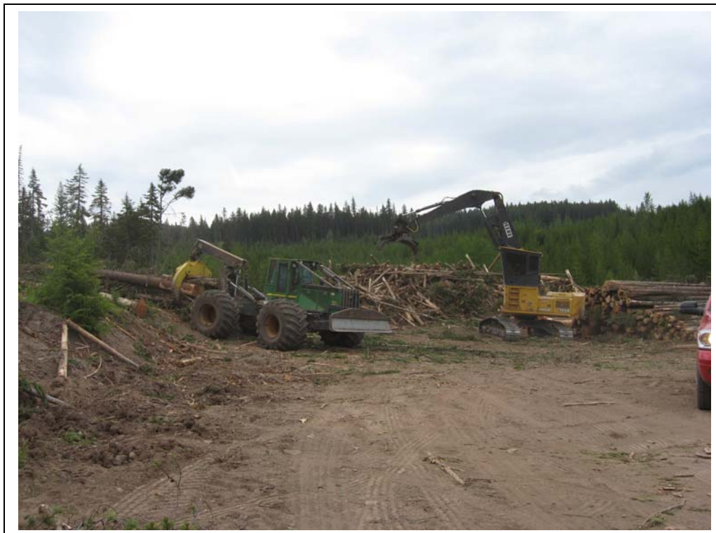
Photo #3: John Deere grapple skidder brings a turn to the landing. The log loader has a butt n top attachment to efficiently sort and deck wood at roadside. The processor will move in to manufacture cut to length logs for the mill. Note the healthy plantation in the background.
